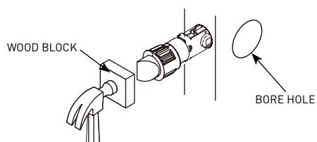
B. Faceplate Latch: Secure to the door edge using latch screws (BB). If it does not sit flush with the door edge, mark an outline using the faceplate and chisel 1/8" (3 mm) deep or until the faceplate is flush.
