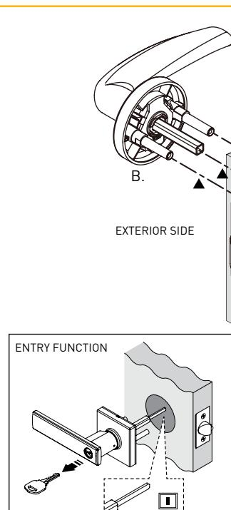
**Note:** To ensure correct alignment of the lever, tighten the mounting screws on the interior lock mechanism while holding the exterior lever upwards.
